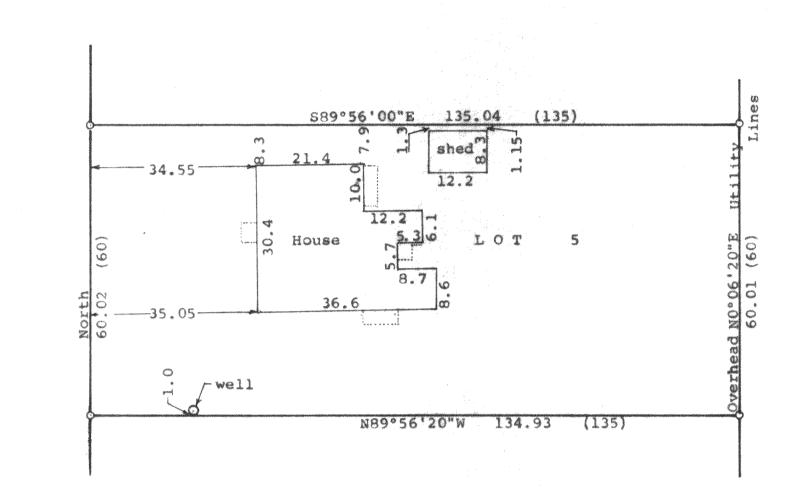
Scale - 1" = 20' •= 1" Iron Pipe Found (0.00) = recorded distance Bearings referenced to the east line of South Shore Drive with the assumed bearing of North Survey ordered by: Century 21, Skandia Realty 312 South 7th street Delavan, WI 53115
